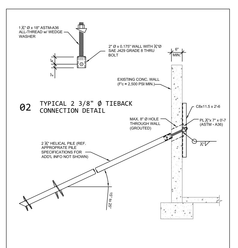
**01** TYPICAL 2 3/8" Ø HELICAL TIEBACK ANCHOR DETAIL
